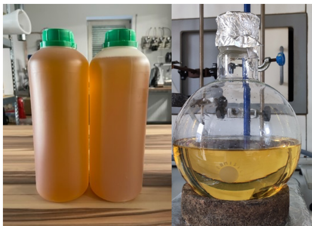
Figure 1. Oils before (left) and after transesterification process (right)
