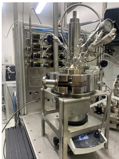
Figure 2. Reactor for transesterification process (left); DSC and STA used for samples characterization (right)
